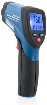
The IRT2 is a handheld, dual laser, non-contact Infrared Thermometer with 12:1 distance to spot ratio and audible and visible high/low set point alarms. It is used to measure and display surface temperatures within the range of -58°F to 1202° (-50°C to 650°C) and has an accuracy of approximately 1 to 1.5% (see Specifications for details). The IRT2 has a fast response time (0.15 sec) and is powered with a 9V battery and complies with Class II UK/EU laser safety standard EN60285.
