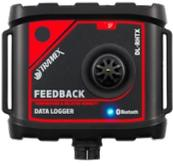
The Feedback DataLogger and App log up to 100,000 data point entries for relative humidity, temperature, dew point and grains per pound, transmitted wirelessly via Bluetooth BLE technology to your mobile device. Used to perform ASTM F2170 with the Tramex Hygro-2 probe.
